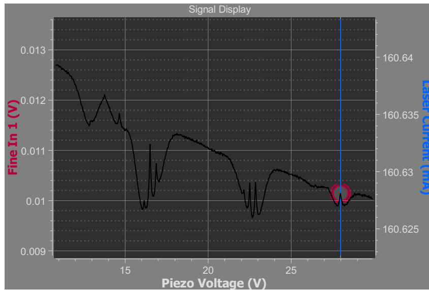
Fig. 11: Here, a lock point is selected from one of the possible lock points. To have a rough indicator for the stability of the frequency, there is a red ball, which moves around at the start of the lock-in process, but stabilizes for the PID settings. Here, the ball has already stabilized at the lock point.
