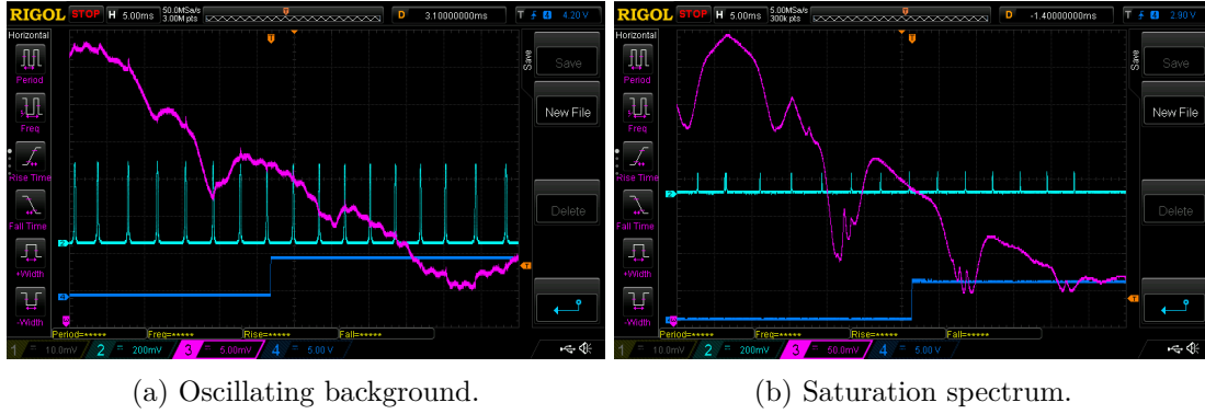
Fig. 9: Saturation spectrum recorded with an oscilloscope. The magenta signal comes from the photodiode, which is placed behind M_4 . a) shows an oscillating background, which needs to be avoided. b) shows, as expected, an underlying triangular ramp with the expected saturation peaks inside absorption dips. The cyan signal comes from the FPI and shows the wanted equidistant structure. The blue square signal is used as a trigger.
