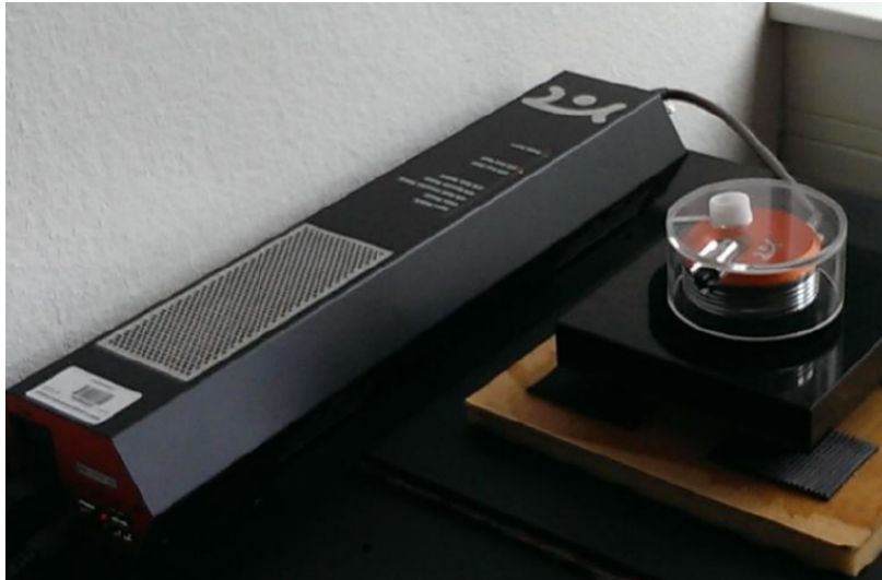
Fig. 7: On the left hand side the electronics of the setup are shown and on the right hand side one can see the scanning head with a sample inside of it. This graphic is taken from [1].
